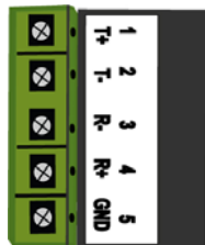
TERMINAL BLOCK WITH 120 OHM TERMINATION
